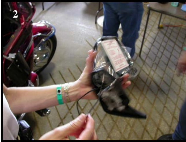
2 Male pins are already installed on harness from Signal ® mirror.
