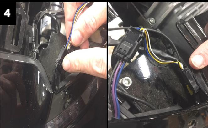
4. Secure and route the windshield trim harness for each side. Route the wires towards the inner fairing. You will notice a small gap at the point where the inner and outer fairing mate. This is where the wires will exit. (shown in Picture 5 and 6)
