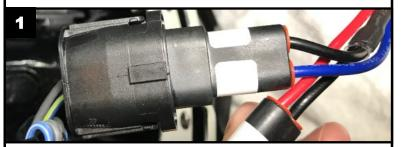
3. Plug the adapter 2 pin **H9** High Beam connector (Red and Black wires) into the bikes headlamp harness High Beam connector (Blue/White and Black wires). See Photo 2.
