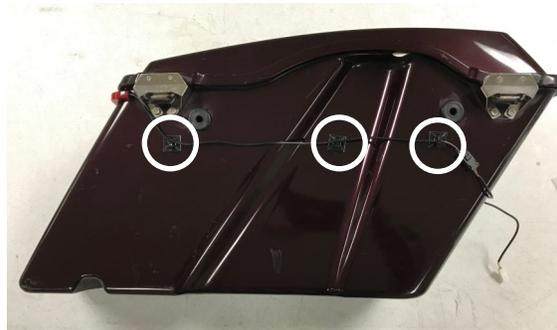
6. Route wires from bag light to each cable tie holder location and secure with enclosed cable ties. Make sure wiring will not come in contact with moving parts or in an area with high heat. Also take care that wires will not get pinched or frayed.
