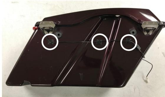
6. Route wires from bag lights to each cable tie holder and secure with tie wraps.
