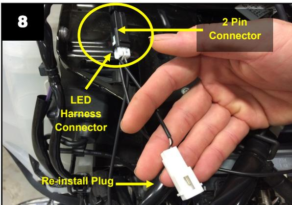
Plug the Vent LED Harness Connector into the fairing 2 pin connector, ensure that it snaps in. Make sure to reinstall the plug removed in step 3 into the LED harness pass-through connector.
