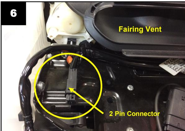
Locate the 2 pin Connector to the lower left (looking at the fairing) of the vent on the motorcycle. See photo, item circled for connector location.
