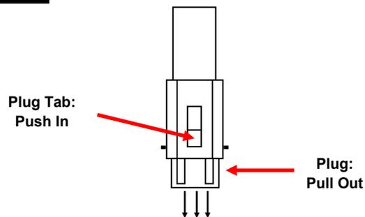
Remove the connector plug from the connector on the motorcycle by pushing the center tab in and pulling the plug out. Save the plug for reinstallation in step 8.
