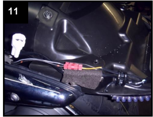
Using supplied Posi-Lock™ connectors from kit install connectors from old turn signals onto turn signal Red leads. (pictures 11 & 12)
