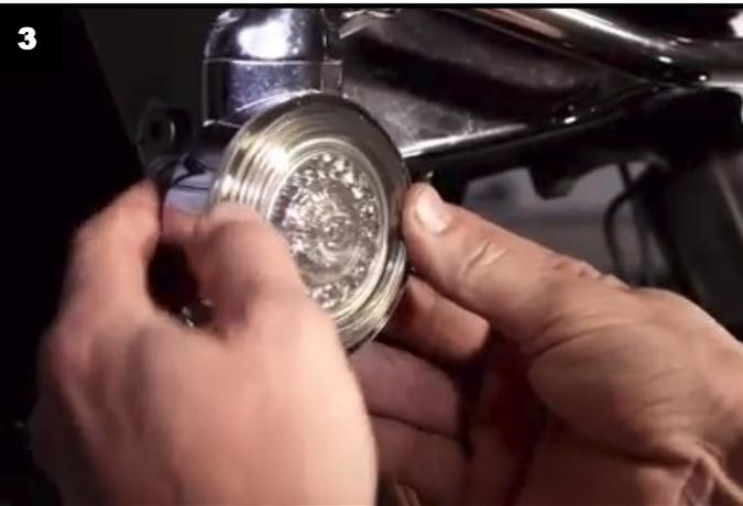
8. Remove the lens and check that adapter is secure, if not remove and adjust tabs and repeat steps 6 and 7. Adapter should be snug but not tight.
