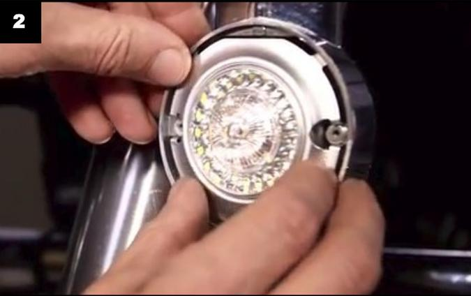
7. Use the Lens to push the adapter into place and fully seat into housing (Figure 3).
