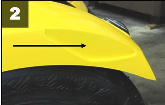
Hold BRIGHTSIDES™ light up to fender noting location where wire meets fender, drill ¼ inch hole in fender for wire to pass through.
