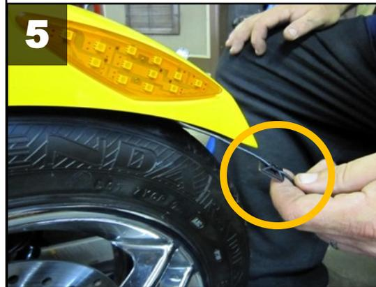
Although shown on the outside the fender in the picture to better show their mounting locations, treat the underside of the fender with the 3M promoter ampule and stick the tie-wrap holders with wire roughly in these areas as shown on the UNDERSIDE of the fender to hold wire in place.
