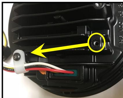
5. Connect the ProBEAM® headlamp to the existing factory H4 plug and re-install according to your vehicle's manual.
