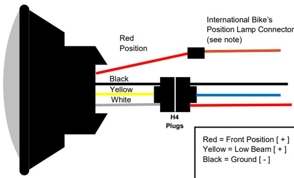
**Note:** The Red (position light or city light) wire is for international applications where a position light illuminated in the headlight is required when parked on a street. It will be connected to the accessory circuit (position lamp connector) of the bike's harness and will illuminate when the ignition is placed in the accessory position.
