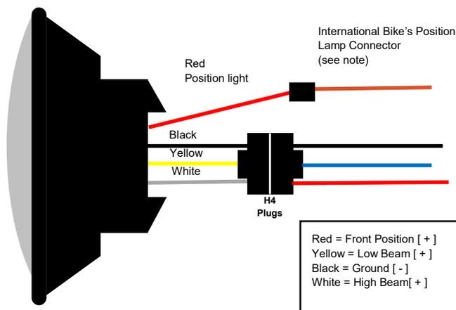
**Note:** The Red (position light or city light) wire is for international applications where a position light illuminated in the headlight is required when parked on a street. It will be connected to the accessory circuit (position lamp connector) of the bike's harness and will illuminate when the ignition is placed in the accessory position.
