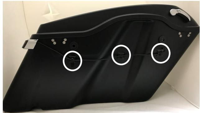
6. Route wires from bag light to each cable tie holder location and secure with enclosed cable ties. Make sure wiring will not come in contact with moving parts or in an area with high heat. Also take care that wires will not get pinched or frayed.
