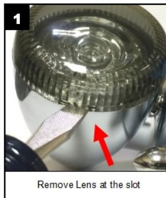
Remove Lens at the slot
