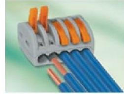
Strip wire 9-10 mm. Use the stripped wire gauge on the back of the connector to verify correct strip length.
