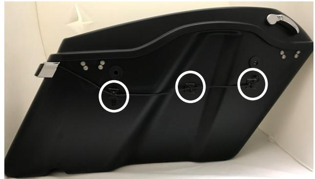
6. Route wires from bag light to each tie wrap holder location and secure with enclosed tie wraps.
