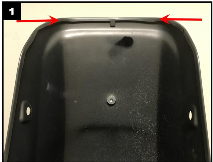
4. Test fit the new Integrated LED Taillight to underside folded lip of the fender. Make sure it is centered, then mark the position with a grease pencil for a guide. **NOTE:** the Integrated LED Taillight mounts on the folded lip of the fender not behind it.
