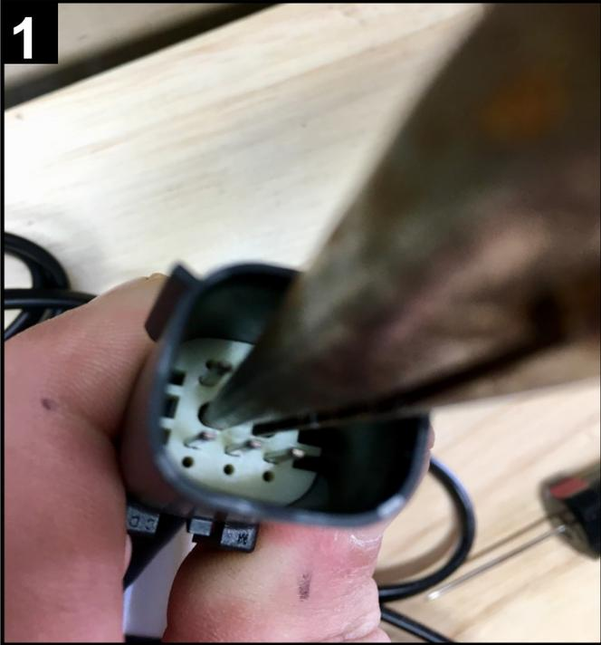
2. Once the secondary lock pin housing is unlocked, insert terminal release tool.
