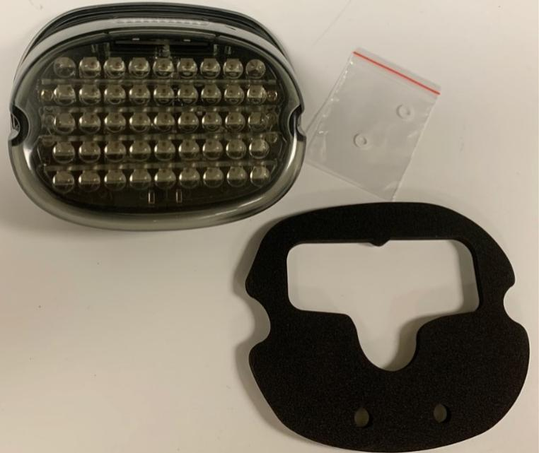
4. Remove white paper from back of gasket and apply gasket to the new LED taillight assembly. (**Note:** Gasket on the new unit will need to make clean contact with the taillight base all the way around.)
