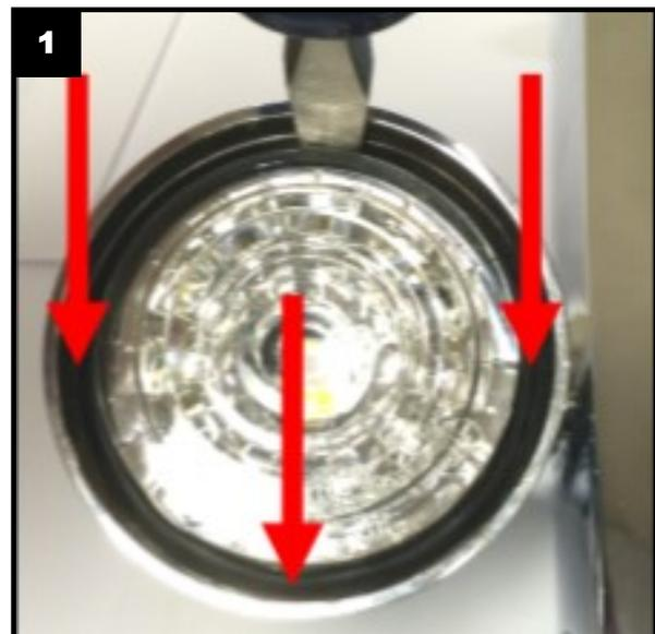
5. Confirm the proper orientation of the socket base and insert the base into the socket. If it seems hard to twist the base in the socket or hard to remove, it is probably orientated the wrong way.
