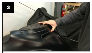
Remove the windshield and front outer fairing from the bike, if unsure of this process, please refer to manufacturer service manual for details.
