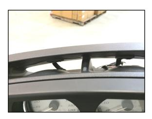
9. Once the LED harness is secured, use the remaining tie-wraps to secure the harness as needed.
