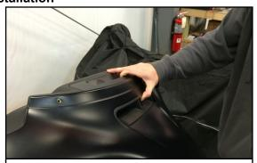
1. Remove the front outer fairing from the bike, if unsure of this process, please refer to manufacturer service manual for details.
