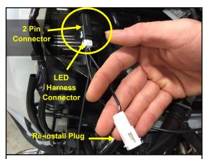
4. Plug the Vent LED Harness Connector into the Fairing 2 pin connector, ensure that it Snaps in. Make sure to reinstall the plug removed in step 3 into the LED harness pass-through connector.
