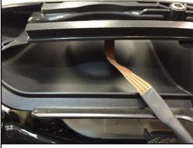
5. Test fit each LED Pad for desired fitment. Notice inside each vent port is a circular cut out in the center. It is ideal to have the LED pad as far into the circle area, yet still allow the vent to open and close.
