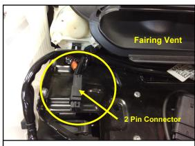
2. Locate the 2 pin Connector to the lower left (looking at the fairing) of the vent. See photo item circled for connector location.
