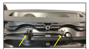
8. Use the Provided Tie-Wrap Bases to secure the LED harness wiring above the Vent. Prime the surface with the adhesive primer and let dry 2-4 minutes before attaching. Once bases are installed, dress wires to fit in the recess then secure with the provided tie-wraps as shown. Leave a little slack in the LED ribbons, so they will lay flat against the vent gasket once the fairing is reinstalled.
