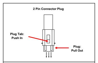
3. Remove the Connector Plug from the connector by Pushing the center tab in and pulling the plug out. Save the plug for reinstallation in step 4.
