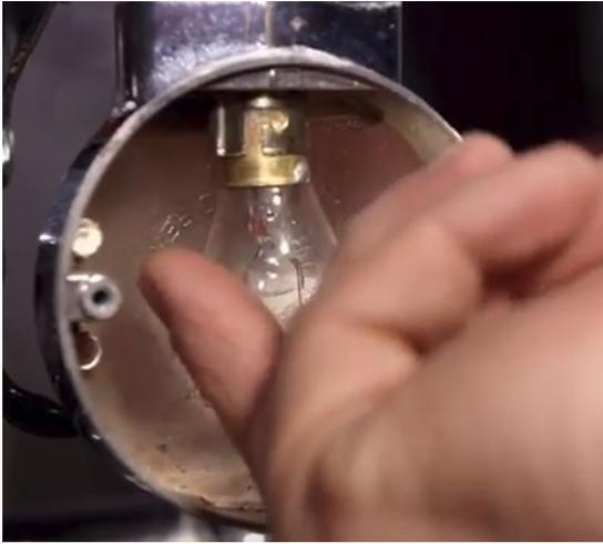
3. Remove any corrosion or dielectric grease from the socket to insure the socket contacts are clean.
