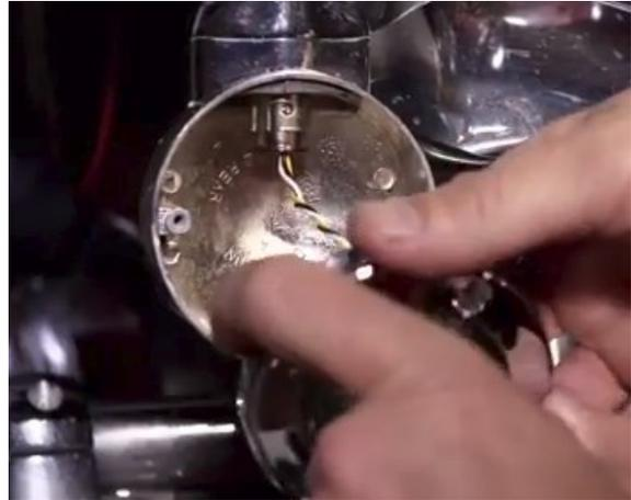
7. Install the Flat Bezel onto the turn signal housing and firmly tighten with the provided screws.
