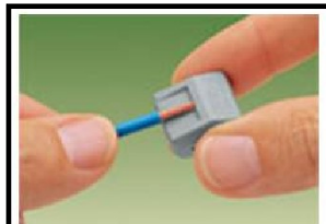
Strip wire 9-10 mm. Use wire gauge on bottom to verify.
