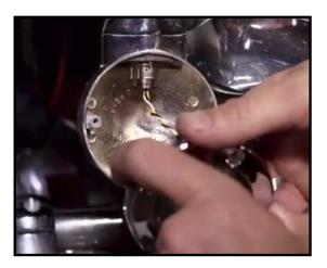
6. Install the Flat Bezel onto the turn signal housing and secure with the provided screws.
