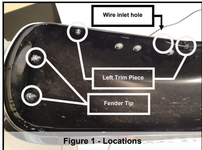
8. Attach the extension cable to the connectors on the fender tip. The Posi-Lock™ connectors twist open, insert wire then twist closed. Make sure Black goes to black and the colored wire goes to red (or colored wire).
