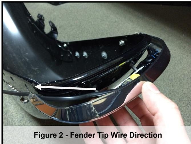
Figure 2 - Fender Tip Wire Direction
