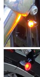
Dual Color 3-wire units function as red brake light on the rear, white running light on the front with full contrast amber turn signal flash. wire leads are equipped with IP68 rated JAE connectors for plug and play installation with Run/Turn Signal Adapters (sold separately).
