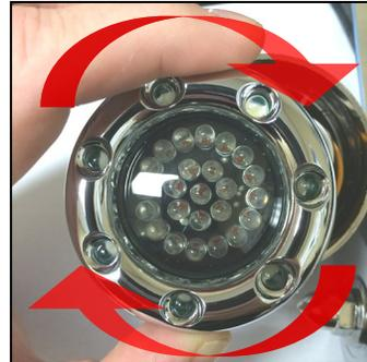
Twist the Ring to coil wire
