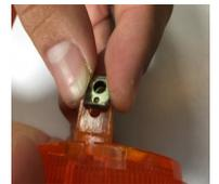
Verify the factory gasket is in place before installing new lens.
