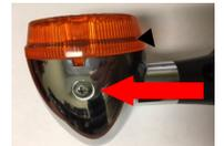
Carefully remove factory lens from housing by applying pressure to the attachment screw side of the lens and pulling out and upwards. Pay attention to the factory gasket ensuring the gasket does not fall out.
