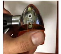
Using your fingers, remove thread clip from the factory lens and install on the new lens.
