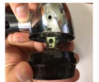
Install the factory mounting screw. Repeat installation for the other side.
