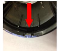
Align the thread clip of the new lens with factory mounting screw hole of the turn signal housing. Press into place until you hear a snap.
