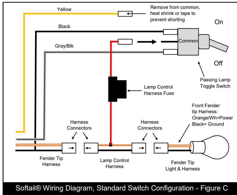
5. Locate the black 2-pin connector containing an ORANGE with WHITE stripe wire and a BLACK wire that goes to the front fender tip light. This connector is located behind the left front side of the fuel tank.
