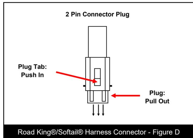
6. Once harness connector is located, unplug the connectors by pushing in the center tab and pulling the male and female sides apart. (See figure D)
