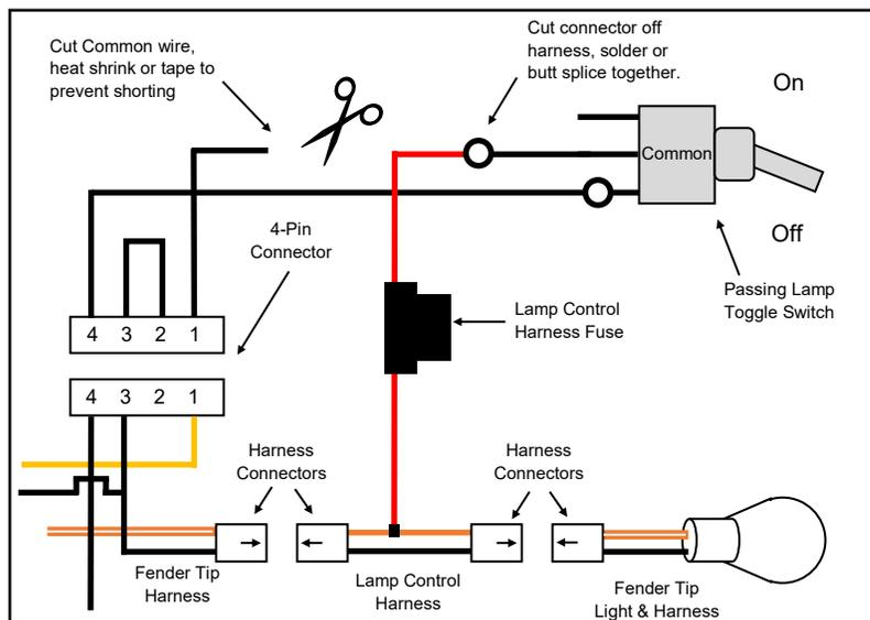
Road King® Wiring Diagram, Switch w/non-removable wiring - Figure B
