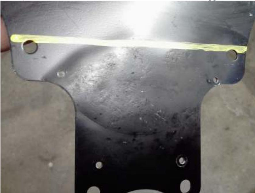
**12)** Center license plate support bracket onto under tail support bracket along reference line and mark the four 1/8 inch holes as shown, We recommend using a clamp to hold the two brackets together while marking to be sure brackets do not move.
