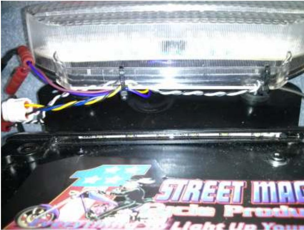
23) Route all wires through hole in left side of under tail cover.
