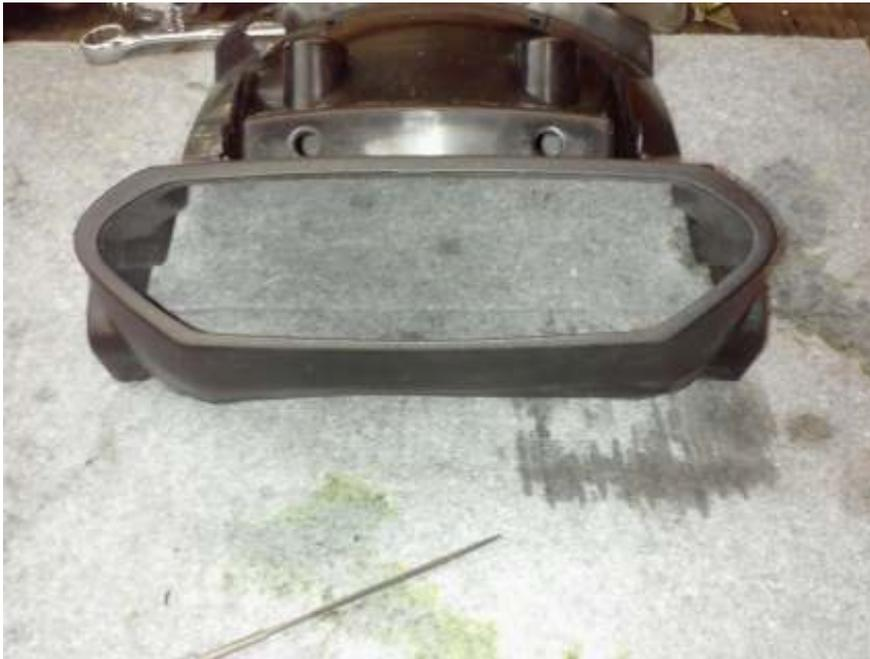
**10)** Using a hammer on a suitable surface pound the under tail support bracket flat in area indicated by yellow lines in photo, once flat bracket should look as shown.
