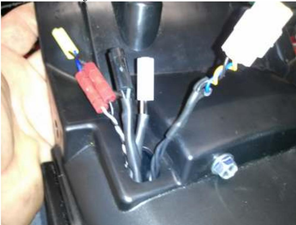
24) Re-plug wires into harness connector coming from bike and reinstall under tail section onto rear fender using the stock hardware removed earlier.
