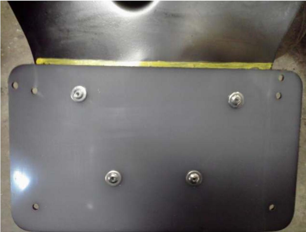
**17)** Mount new Street Magic Integrated Tail Light on to under tail support bracket using original tail light hard ware.
